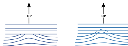
Figure 3-42. How contour lines represent overhangs.
